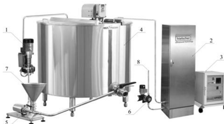
Fig 2. Industrial version of implementation: 1 - rotary dispersant; 2 - sonochemical reactor with generator 3; 4 - mixing tank; 5 - circulation pump; 6 - metering pump; 7 - a device for the introduction of dry skim milk; 8 - water inlet
